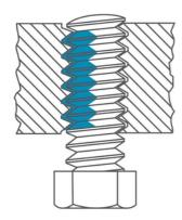
Tuflok<sup>®</sup> patches are well known for their cost benefits. They allow the same screw to be reused a number of times. As a result, maintenance and disassembly operations are simplified and cheaper.
