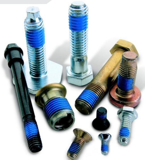
The radial tension created by the elastic deformation of the product causes position retention through increased friction. The parts that are retained can be repositioned as the nylon deformation is partially reversible so that part can be screwed down and unscrewed several times. The retaining function is immediately active once screwed down.
